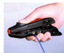
压接时用大拇指向前推即可 Push forward with thumb when crimping
