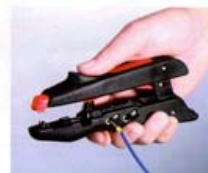
根据管形端子的大小选择压接口 Select clamping nozzle according to the size of pipe terminal
