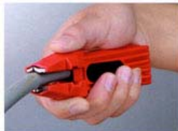
剥离护套的电源线 25mm 2 以下 To strip the power cord with sheath under 25mm 2
