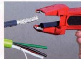
用于同轴电缆的导线剥皮 For the stripping the conducting wires of coaxial cables
