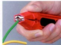
剥单芯电源线。剪断电源线 Stripping power cord with single core, Cutting power cord
