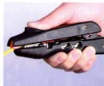
用大拇指按住向前推 Press down with thumb and push ahead.
