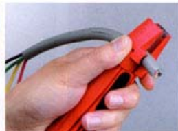
纵向剥带护套电源线 Longitudinally stripping and cutting power cord with sheath
