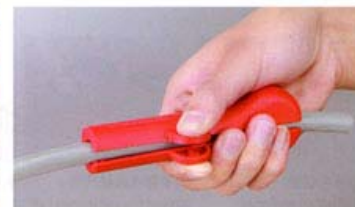
双壳体叠合式剥皮工具 Double-shell laminated stripping tool
